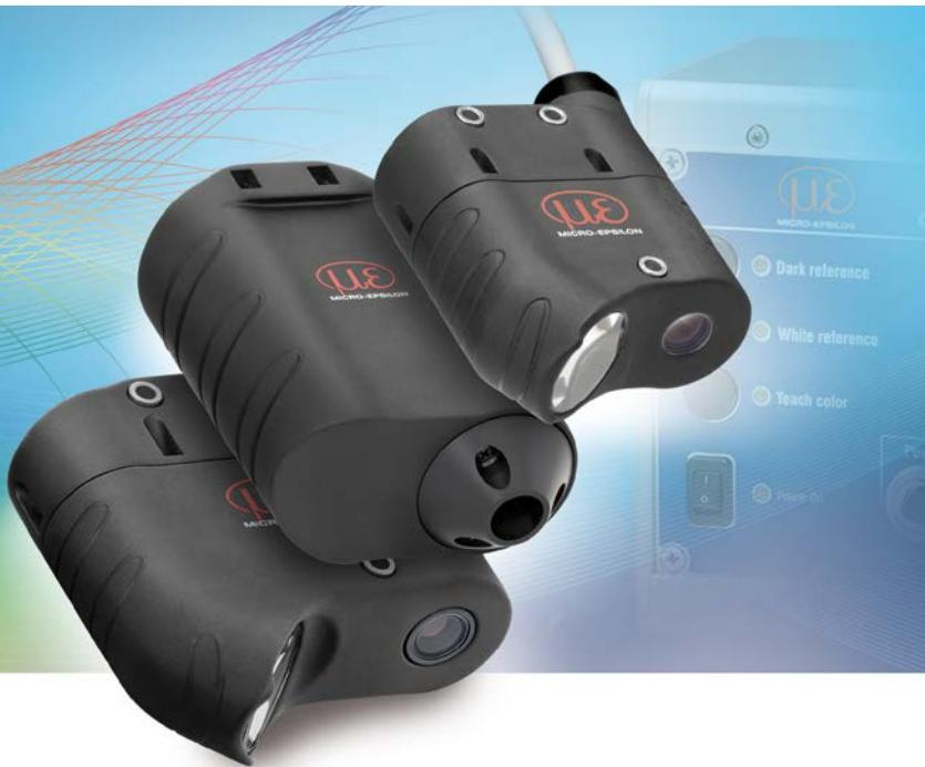
The standard sensor ACS1 is used for common measuring tasks. The transmitter and the receiver inside the sensor are arranged at an angle of  $45^\circ \times 0^\circ$  or  $30^\circ \times 0^\circ$  to each other, producing a working distance of 38mm or 50mm.
